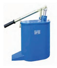
Hand pump type 10-2400 is applied for charging other pumps in small lubrication systems. The pump design is based on the principle of a double - acting piston. It is of simple design suitable for carrying. The pump is equipped with tank for lubricant. The proper flexible hose can be added on request.
